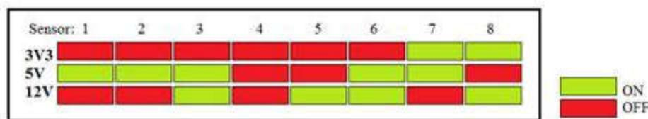
Fig. 1. Visual representation of programmable key
