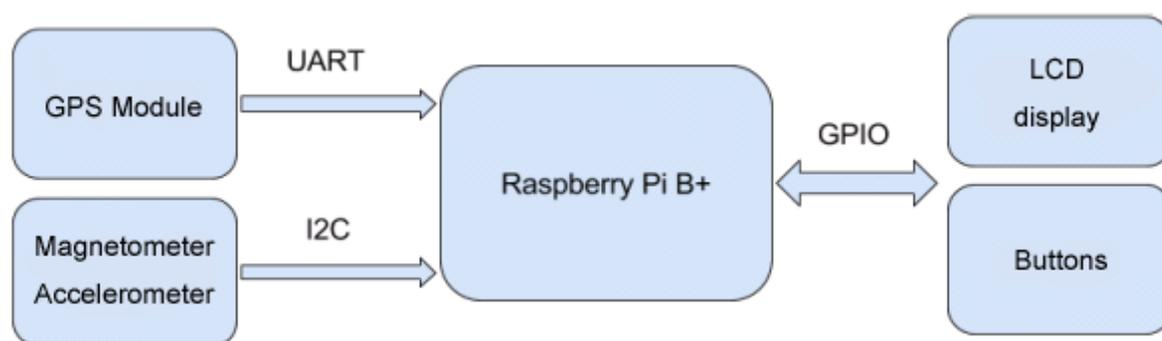
Fig. 1. The block diagram of the computer for car
