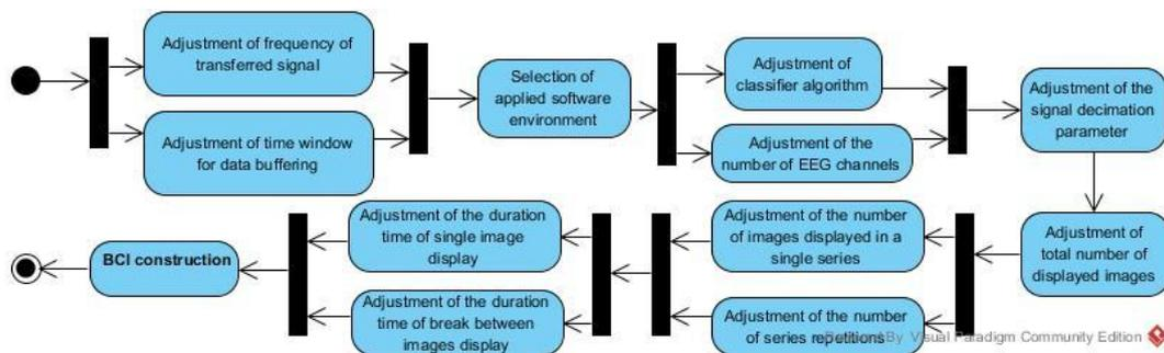
Fig. 2. The procedure of parameters adjustment
