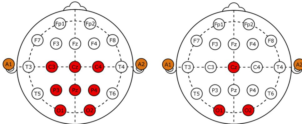
Fig. 1. The scheme of eight (left) and three (right) electrodes placement
